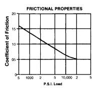
The low friction characteristic of the Duralon bearing is due to the Teflon fabric liner. Increased loading, at constant speed, results in a marked decrease in the coefficient of friction.
